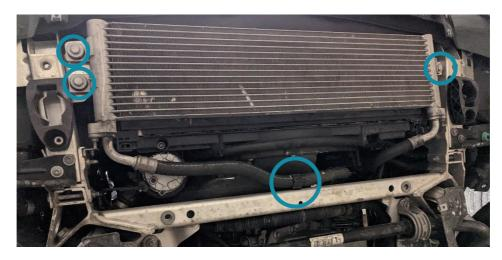
8. Next remove the 2x T25 bolts holding the fan shroud extension and unclip the hose from the fan:
