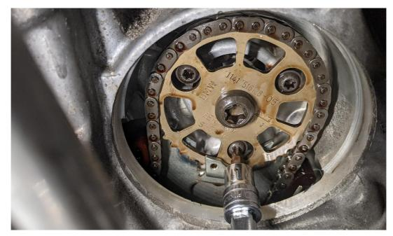
37. Now using a flat head screwdriver, very carefully depress the timing chain tensioner (pictured on the left below). Hold the screwdriver in place and then slide the timing gear off the tip of the Vacuum pump shaft. Once the gear is off the shaft, release the screwdriver and allow the gear to rest as pictured (right):
