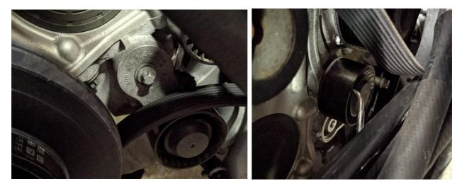
The first pulley (above left) can be removed via the single E12 bolt. The second pulley (above right) first needs the plastic cover popped off, and then the T50 bolt removed. You may need to rotate the oil cooler lines slightly to get access to the T50 bolt.
