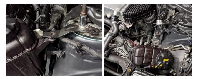
25. It's now time to remove the intercooler. The intercooler outlet clamp and both charge pipe clamps can be loosened using a 6mm nut driver. Next, unplug the map sensor and remove the coolant hoses as pictured below. You may want to place rags under the coolant hoses upon disconnecting for any residual fluid.
