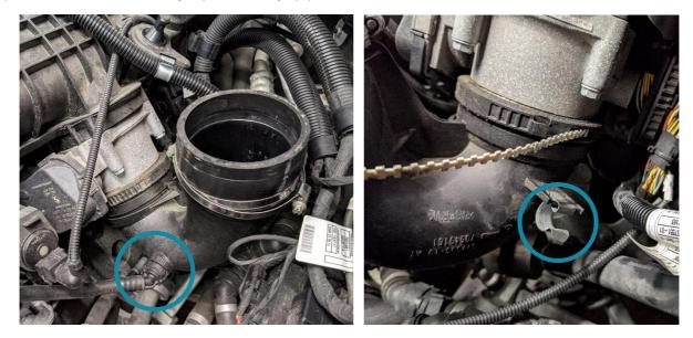
27. Prepare to remove the intake manifold by removing all electrical connections, clips, etc. that will be in the way. This includes the oil pressure sensor plug, rail pressure sensor plug, MAP sensor plug, and rear manifold bracket (2x T25 bolts pictured below, right).
