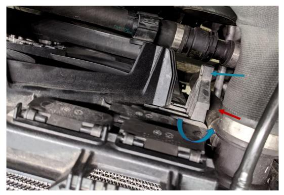
The left side fan mount actually pivots 90 degrees once it's moved into a location to do so. It is somewhat difficult to move, but it "snaps" into a 90 degree position (pictured). You will need it in this clocked position and it needs to be inside the hose (red arrow) as pictured. This will allow for the removal of the fan through the bottom of the car.
