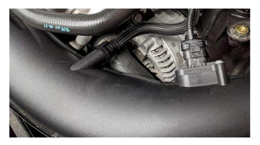
Loosen the hose clamp using a 6mm nut driver and pull the coolant hose out of the clips as pictured. To remove the front clip, first turn the rubber grommet ¼ turn and then squeeze the clips inward and push down.
