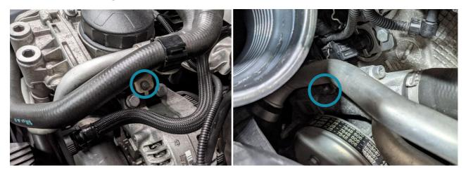
15. At this point the fan is free and the removal process can begin. To start, the fan needs to be lifted slightly out of its lower and side brackets and moved slightly to the left. This is to gain clearance for the pivoting mount:
