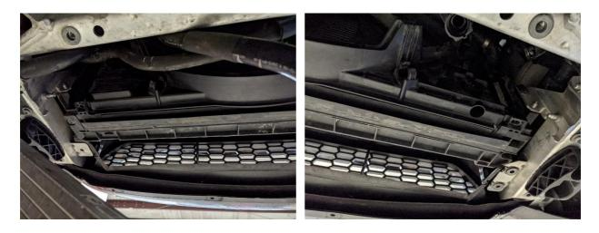
12. Now, moving up top, remove the hose clip from the fan assembly on the left side:
