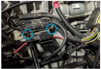
The low pressure line (17mm nut side) can now be disconnected from the pumps and leaned over out of the way for vacuum pump removal. The high pressure lines can be removed entirely.
