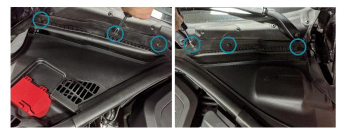
The is also a plastic clip on the outside edge of each cowl cover. Remove this by pulling out the center first, and then the base:
