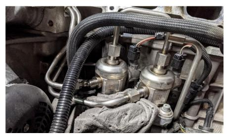
33. Now loosen the low pressure hardline hold-down clamps. Remove the two 13mm bolts below the cable junction assembly:
