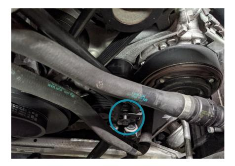
18. Using a T60 socket, rotate the serpentine belt tensioner clockwise and remove the belt from the AC and Alternator pulleys. Take note of the belt routing before removal.
