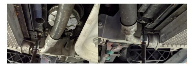
7. Next remove the oil cooler and let it hang freely out of the way. To do this, unclip the hose from the subframe and then remove the 3x 13mm bolts:
