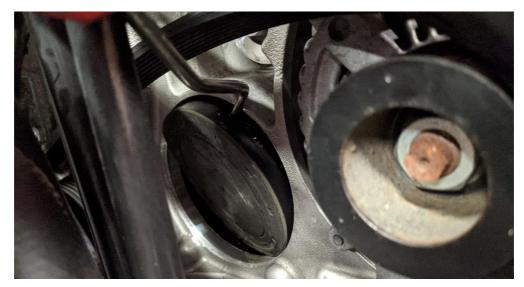
The above sealing cap was finished off with hand tools. By leveraging the bottom in further with the hook, the top edge of the seal became exposed. Once exposed, a long flathead screwdriver and hammer were use to tap downwards on the exposed edge of the seal. This allowed enough rotation to then get the hook in the top (pictured above). Once the top is out, the seal pulls right out.
