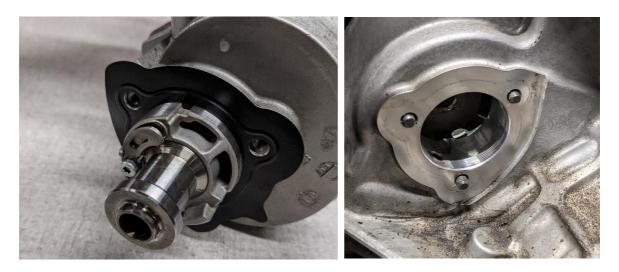
42. The Dorch Engineering vacuum pump assembly can now be installed in the block. Once it is seated in place, the timing gear needs to be placed back on the front of the shaft (reverse process of Step 37). This will require carefully using a screwdriver (again) to hold back the timing chain tensioner while the lining up the gear onto the front of the shaft.
