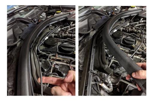
3. Remove the ECU cover by first unclipping the coolant line and then pulling directly up on the cover:
