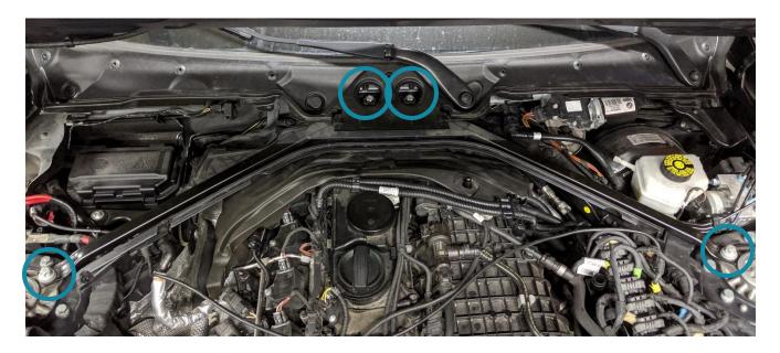
7. Next remove the seven 10mm bolts holding on the upper firewall plastic shroud. There are four bolts on the left side and three on the right:
