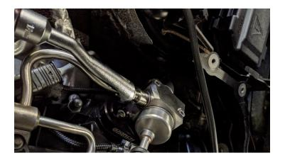
High Pressure Line Nut Tightening Torque: 31nm
