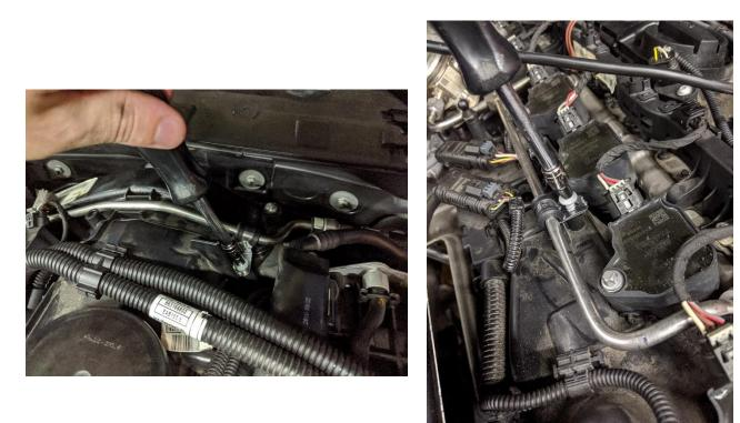
12. The high pressure line can now be completely removed, but **DO NOT SPILL** fuel on the coil pack boots.
