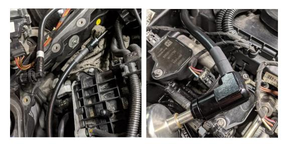
Once the collar is fully threaded, use a wrench to snug the collar. You may need to hold the hose in place by using an additional wrench on the hex portion of the hose fitting.
