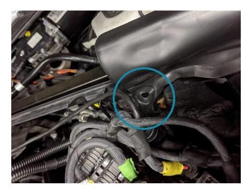
5. To gain access to the strut bar bolts under the cowl, remove the two black circular covers pictured below. These can be removed by reaching underneath and pushing out from the center. Place a hand over top of them as they are pushed out so they don't fly out and get lost.
