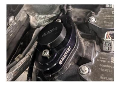
16. Now remove the alignment tool and insert the Dorch Engineering fuel pump. Use extreme **CAUTION** when installing the pump. The bolts MUST BE TIGHTENED EVENLY. Uneven loading of the spring can damage the pump. Also, be **EXTREMELY CLEAN** as all HPFPs are very sensitive to contaminants.
